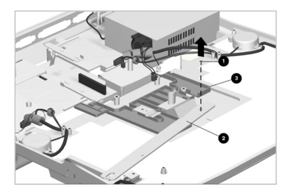
Figure 6-31. Disconnecting the Docking Bar from the Puller Plate
